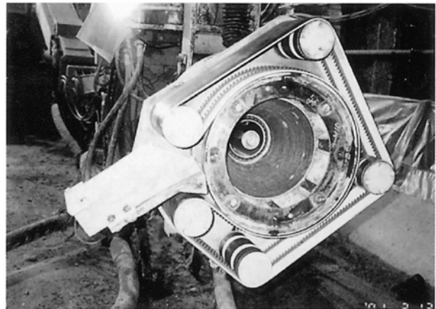
Figure 3: Appearance of centrifugal head with impeller wing and stirring bars removed.
