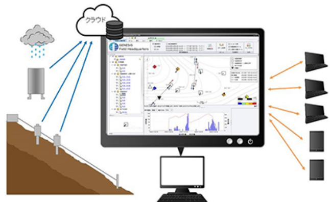
GENESIS/FHQ, a ground behavior monitoring system
