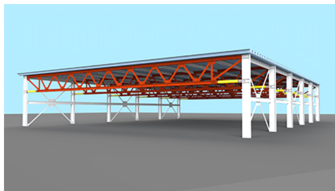
Damage control type truss beam construction method RAIJIN™
