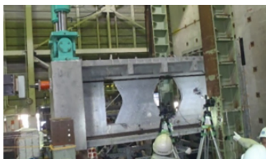
Shear strength testing of joints
