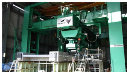
Driving testing with wheel loads on floor slabs
