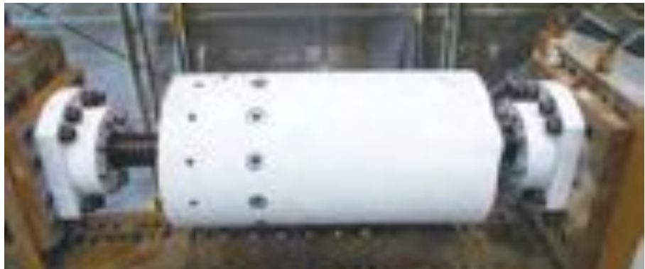
Rotary damping tube (RDT) as attenuation equipment with amplification mechanism
