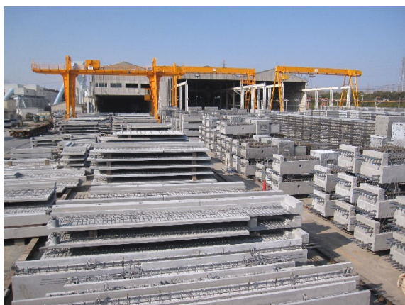
【PCa parts stored in the factory after manufacturing】
