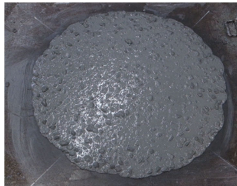
★ High fluidity Example of slump / slump flow measurement Top: Conventional high-strength concrete Below: Sustain - Crete™
