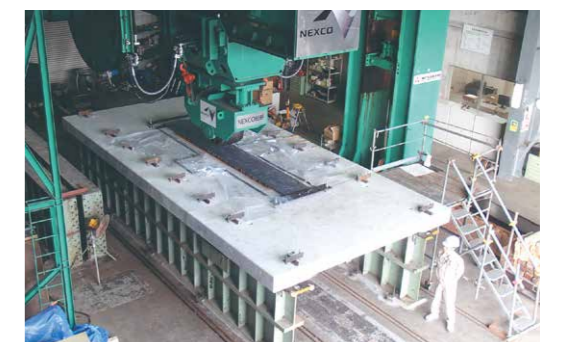
Photograph of specific achievement: floor slab wheel load test
