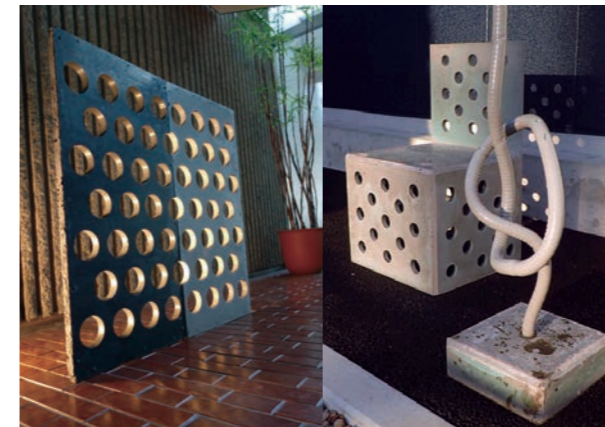
Forms produced with Sustaincrete
