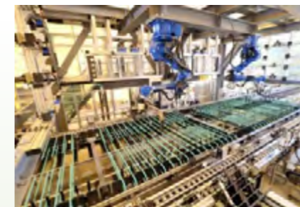
Image of reinforcement assembly for PC floor slabs (Notogawa Plant)
