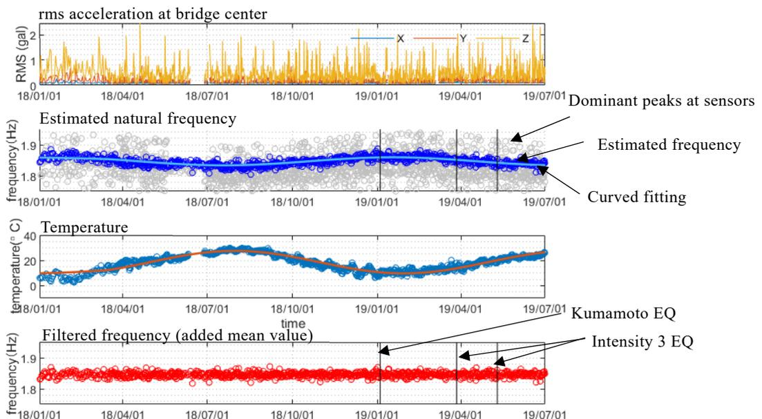
Fig. 8. 2<sup>nd</sup> vertical mode frequency variation and anomaly detection in the Terasako Choucho Bridge
