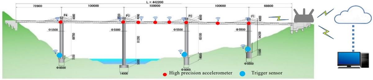
Fig. 3. Monitoring system in the Mukogawa Bridge
