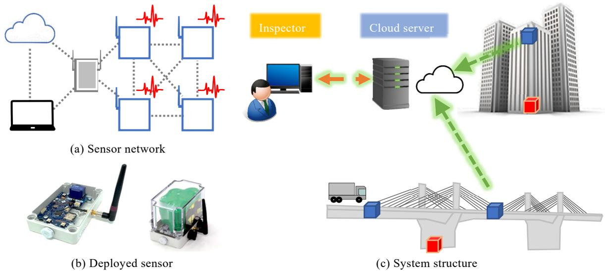
**Fig. 1.** Concept of wireless sensor network monitoring
