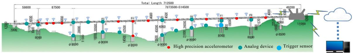
Fig. 4. Monitoring system in the Terasako Bridge
