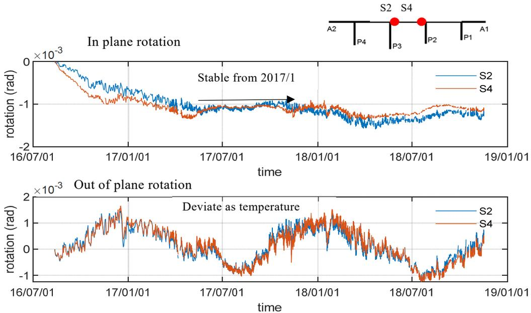
Fig. 7. Inclination variation in the Mukogawa Bridge
