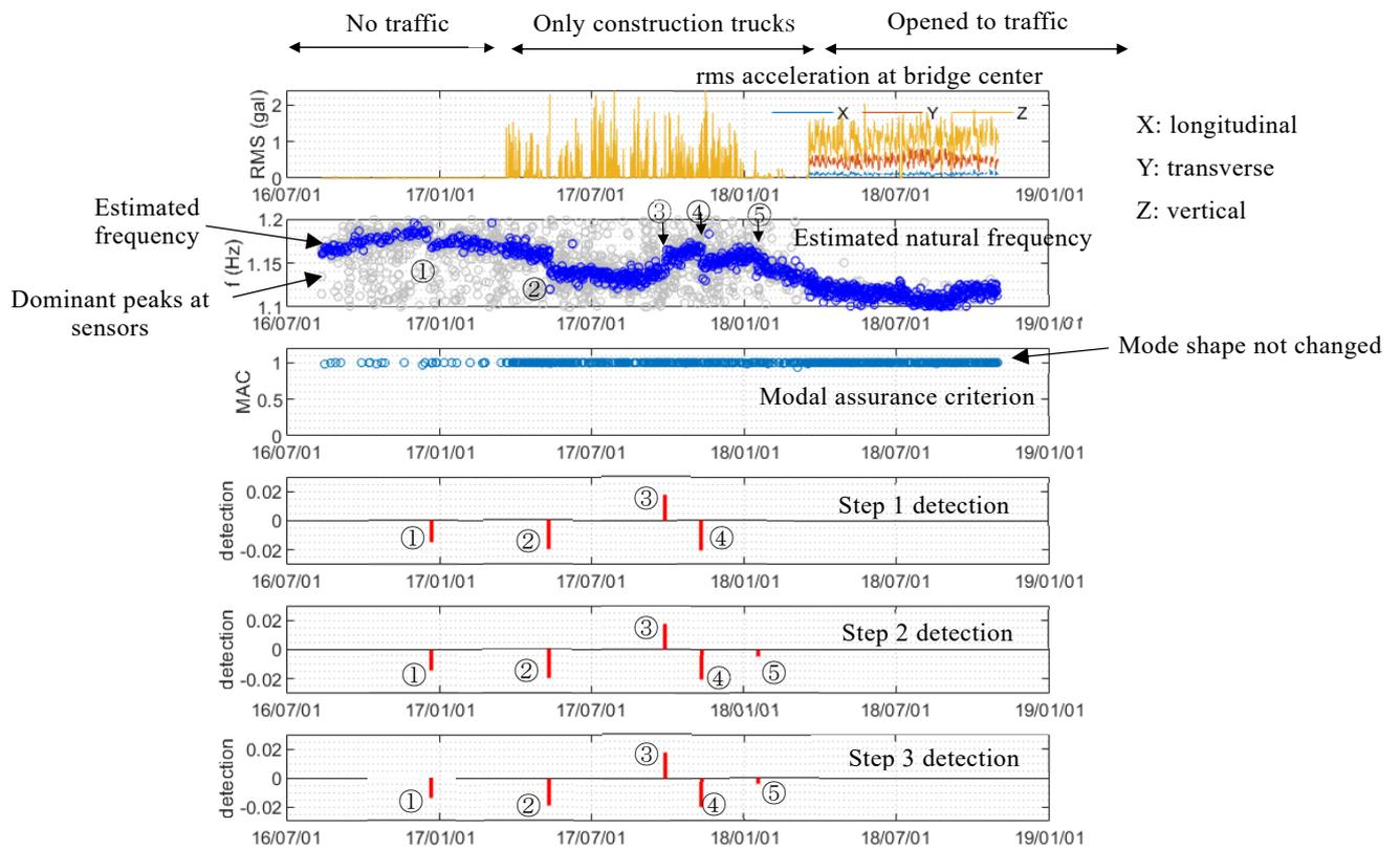
Fig. 12. 1<sup>st</sup> vertical mode frequency variation and anomaly detection in the Mukogawa Bridge
