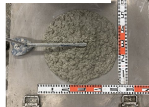
4) No.9 NC27.5-50 (W/B=27.5% BF 置換率 =50% Ad=B×0.80%)
