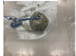
2) No.3 NC42.5-50 (W/B=42.5% BF 置換率 =50% Ad=B×0.75%)
