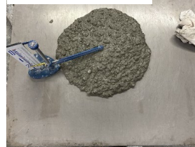
3) No.7 NC27.5 (W/B=27.5% BF 置換率 =0% Ad=B×1.05%)
