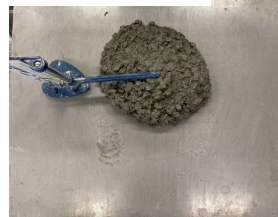
1) No.1 NC42.5 (W/B=42.5% BF 置換率 =0% Ad=B×0.90%)
